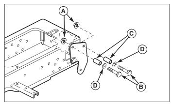
Figure 2. Install Rear Spacers
